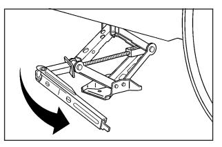
11. Lower the vehicle by turning the jack handle counterclockwise.
